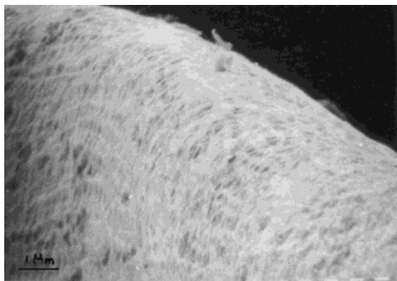
Figure 8 Scanning electron micrograph of silane-treated OPEFB fiber surface ( \times 400 ).
